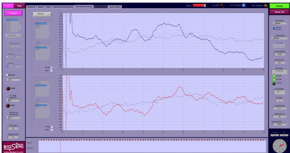
Figure 12a – ERP Tab – ABR building up – screen shot taken (new in the ERP Tab allows saving of both; either stopped or running acquisition) after 1962 sweeps (The image shows a grey and two-colored traces – the grey trace shows that there is little noise as it is quite flat)
