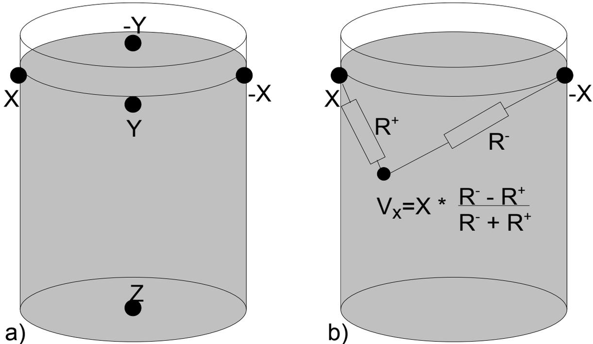
Figure 1: a) positions of the electrodes that inject the current in the fluid (grey) filled container. b) the amplitude of the signal depends on the relative distances to the current injecting electrodes. Lower in the container the resistances are more similar and the amplitude of the recorded signal increases less with the distance from the center.
