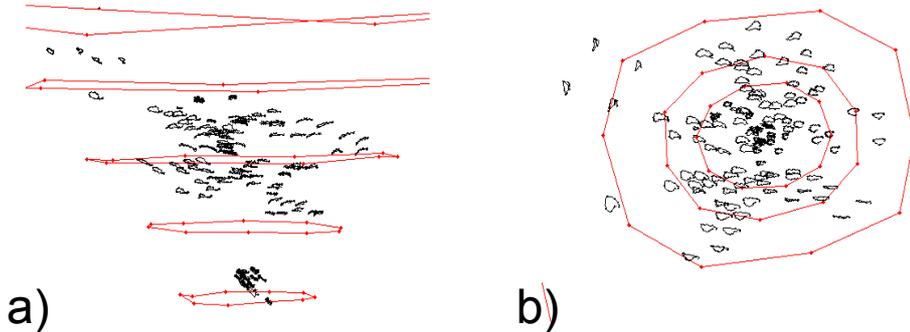
Figure 3: a) front view of the electrodes. In red and drawn lines the electrodes on the inside of the container. In black the needle electrodes moving during one heartbeat. Note that the container appears distorted with the radius of the container ('surface') electrodes near the bottom much smaller than those at the top rows. b) top view.
